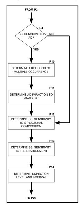
Figure 2-4-4.4. Accidental Damage and Environmental Deterioration (Non-Metallic) Logic Diagram
