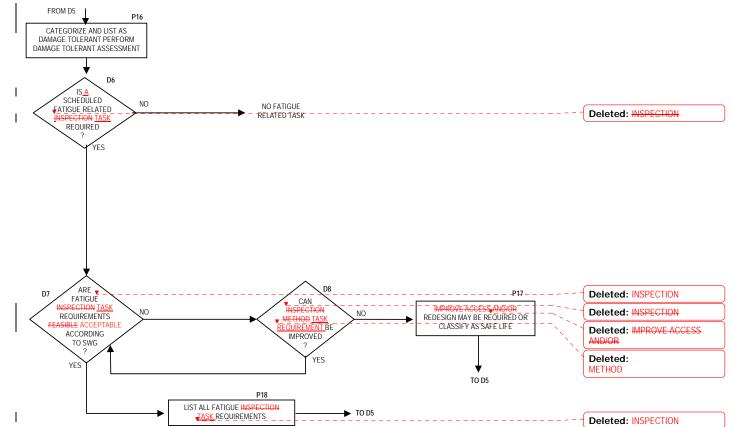
Figure 2-4-4.6. Fatigue Damage Analysis Logic Diagram
