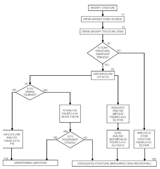
Figure 2-4-4.1. Structural Logic Diagram
