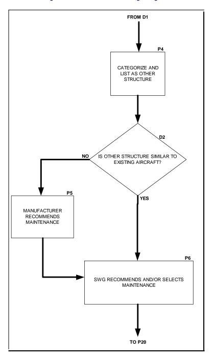
Figure 2-4-4.2. Other Structure Logic Diagram
